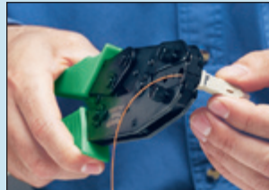
Step 6: Crimp the connector
