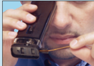
Step 6: Crimp the connector
