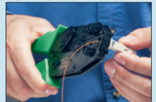
Step 6: Crimp the connector
